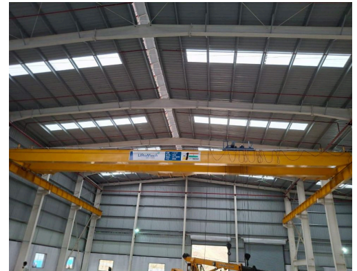
LiftoMech double girder bridge with crab on girders
