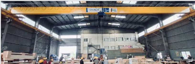
01 EOT Cranes • Single Girder Efficient single-girder overhead cranes for standard-duty lifting inside plants and warehouses.
