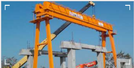
04 Goliath • Gantry Rail-mounted outdoor gantry cranes for yards, precast & material handling.
