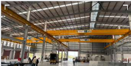
02 Double Girder EOT Higher-capacity, higher-headroom cranes for heavy production environments.
